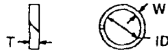
Chart 2B-1 SINGLE-TURN BACKUP RINGS FOR USE WITH GLAND O-RINGS IN MIL-H-5606 AND MIL-H-83282 HYDRAULIC FLUIDS
