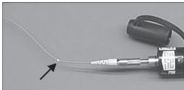
Figure 8. Fault Finder and an Illuminated Break in a Fiber
