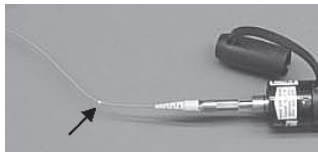
Figure 2. Fault Finder, Light Leakage Through Cable Jacket
