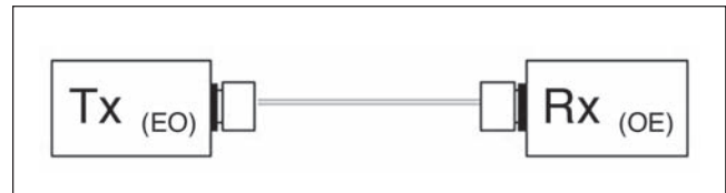
Figure 1. Simple Fiber Optic Link
