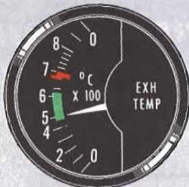
EXHAUST TEMPERATURE J57-23 ENGINE AF 53-1791 THRU 55-3464
