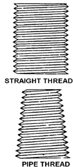
Figure 5. Straight Thread and Pipe Thread
