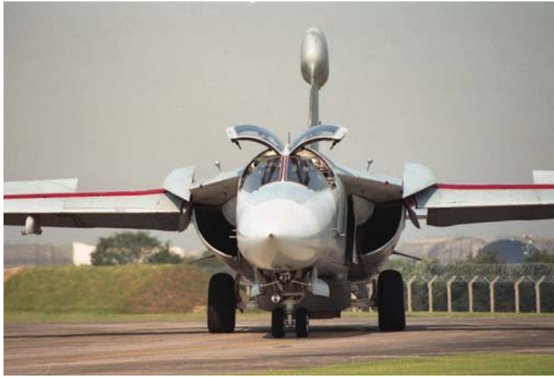
EF-111A 66-037 shows the plethora of additional antennas needed for its job, the unique, robust undercarriage structure and the distinctive 'aardvark ears' canopy sections. This was the first EF-111A for the 42nd ECS, and it completed 49 missions during Operation Desert Storm . (Author)
