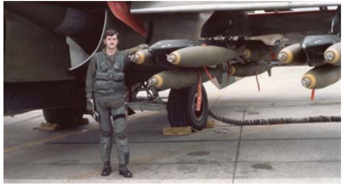
WSO Capt Richard B. Tourtellot and a full load of Mk 82 low-drag general purpose (LDGP) bombs, ready for another Constant Guard V mission. This ordnance replaced the bomb-load of four Mk 84 2,000lb LDGPs after several of the latter armed themselves immediately after leaving their pylons at low altitude, possibly causing otherwise unexplained losses. (Lee Dodd)
