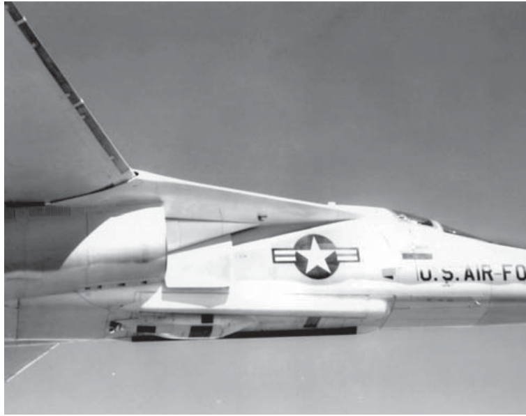
F-111A 63-9776, the only RF-111A, tested the advanced reconnaissance pallet, fitted into the standard weapon bay, between December 1967 and October 1968. Reconnaissance versions of both the F-111A and F-111B were originally required, amounting to 305 examples in all. This F-111A was the last Aardvark with conventional ejection seats. (General Dynamics)
