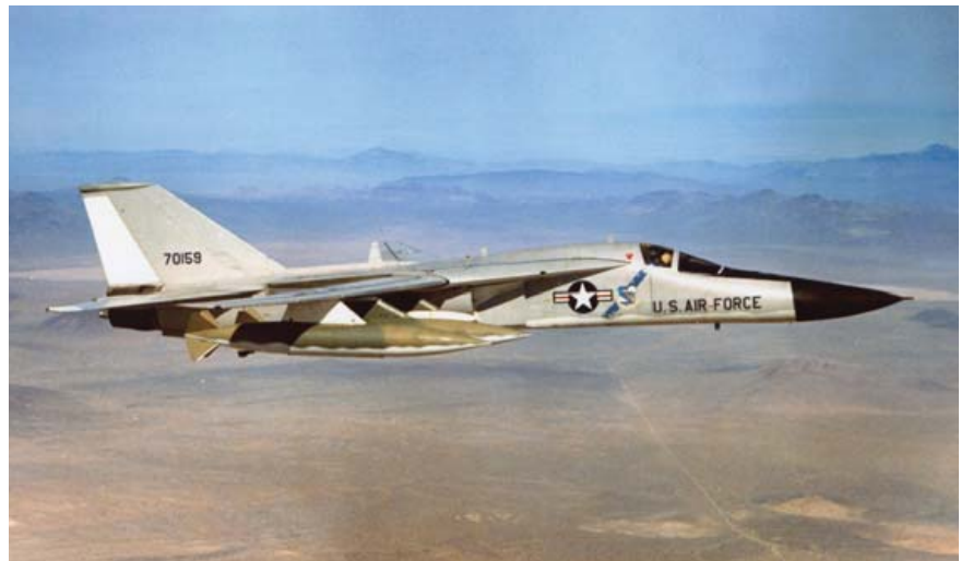
The first FB-111A, displaying Triple Plow I intakes, a SAC 'Milky Way' sash, 600 US gallon external tanks and a nuclear 'shape'. Delivered to the USAF on 30 August 1968, it was employed mainly on test work at Sacramento Air Logistics Center until November 1991. (General Dynamics)
