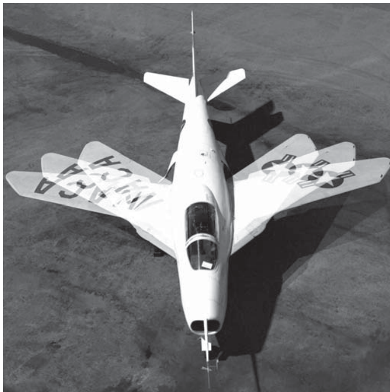
Bell's two X-5 prototypes (50-1838 and 50-1839) began to test variable-sweep wings on 20 June 1951 at Edwards AFB, using the roller-and-rail wing 'translation' mechanism for the first time on 27 July. (USAF)
