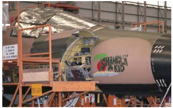
Avionics bays occupied the internal area between the radome and the crew module, accessed through lift-up doors. F-111E 68-0035 of the 55th TFS is seen here undergoing programmed depot maintenance. Its nose-art began with the 'Shamrock Kid' name and shamrock leaf in August 1987. The tropical island was added by February 1988. (Author)
