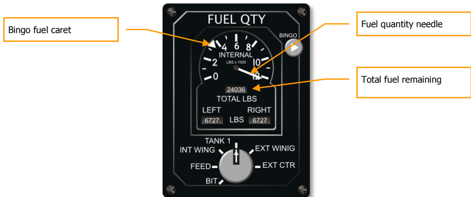
Figure 35. Fuel Quantity Indicator
