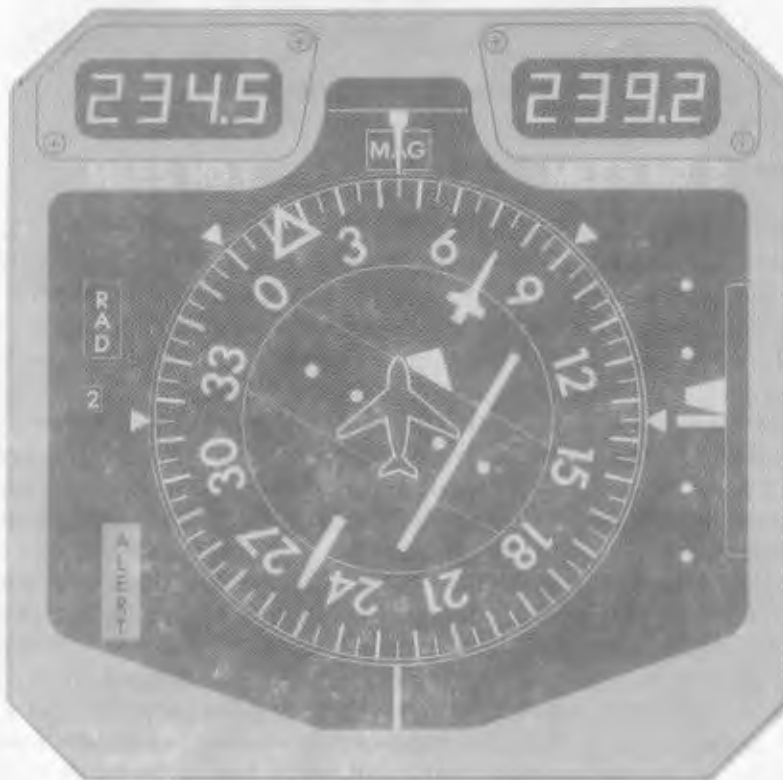
Figure 2-10. 331A-8A Horizontal Situation Indicator.
