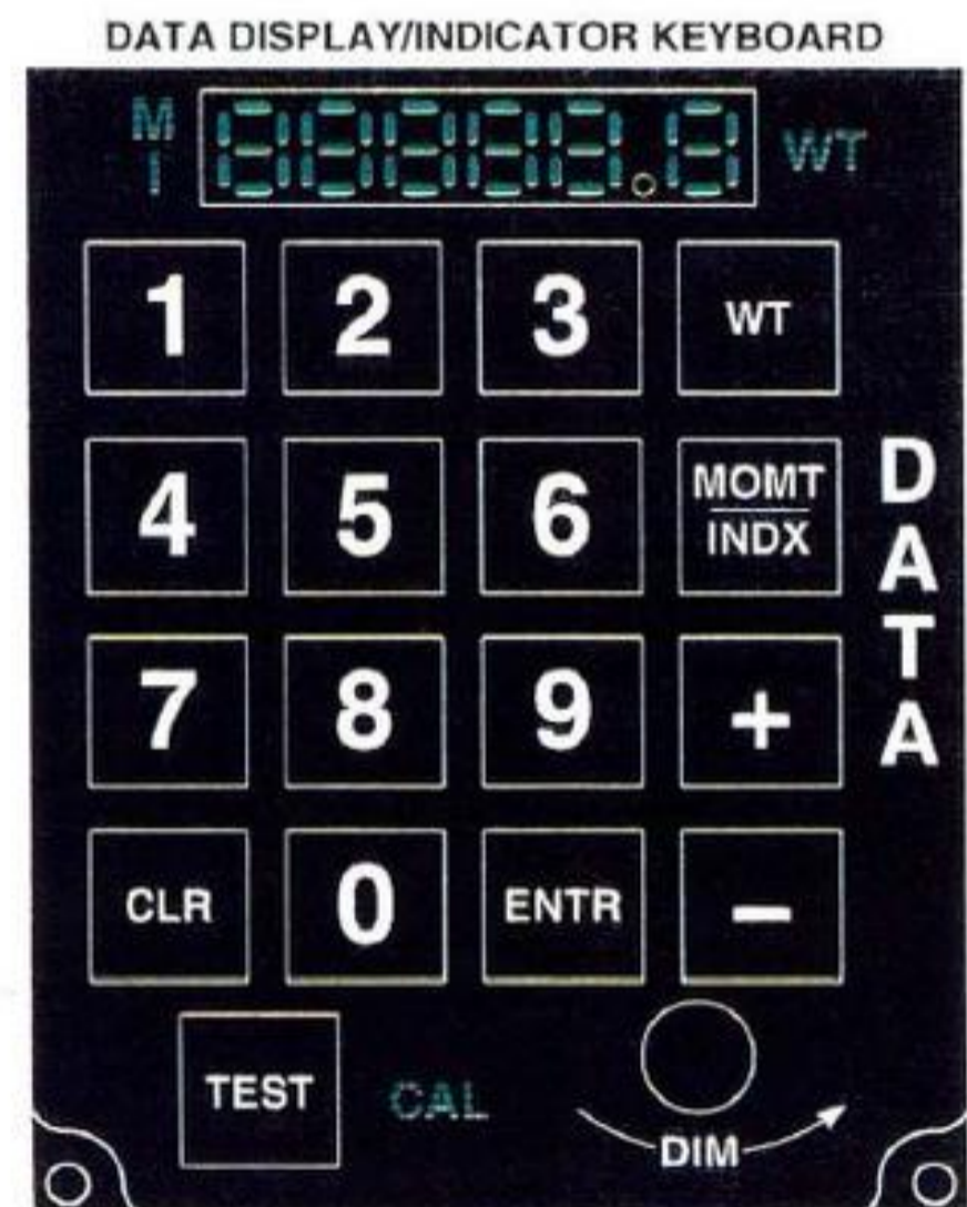
Figure 2-34. CG/Hook Load, Data Display/Indicator/Keyboard
