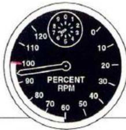
GAS GENERATOR TACHOMETER
