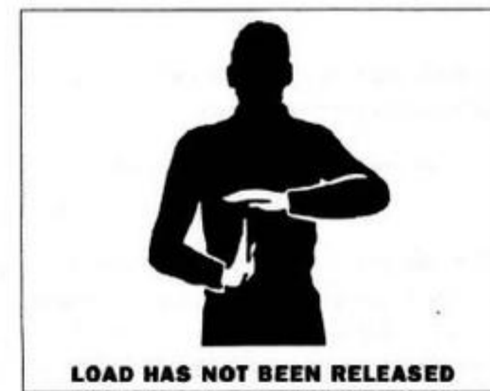
Figure 9-11. Hand and Arm Signals for External Lifts (Sheet 2 of 2)
