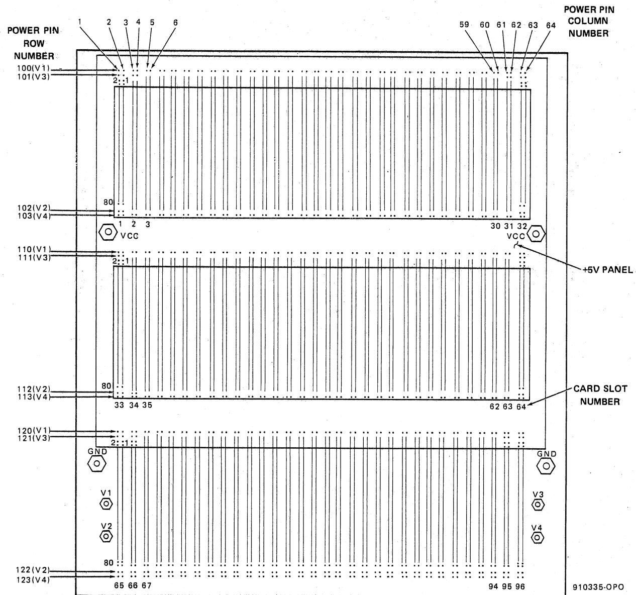
Figure 1-1. Backpanel Card and Pin Numbering System.
