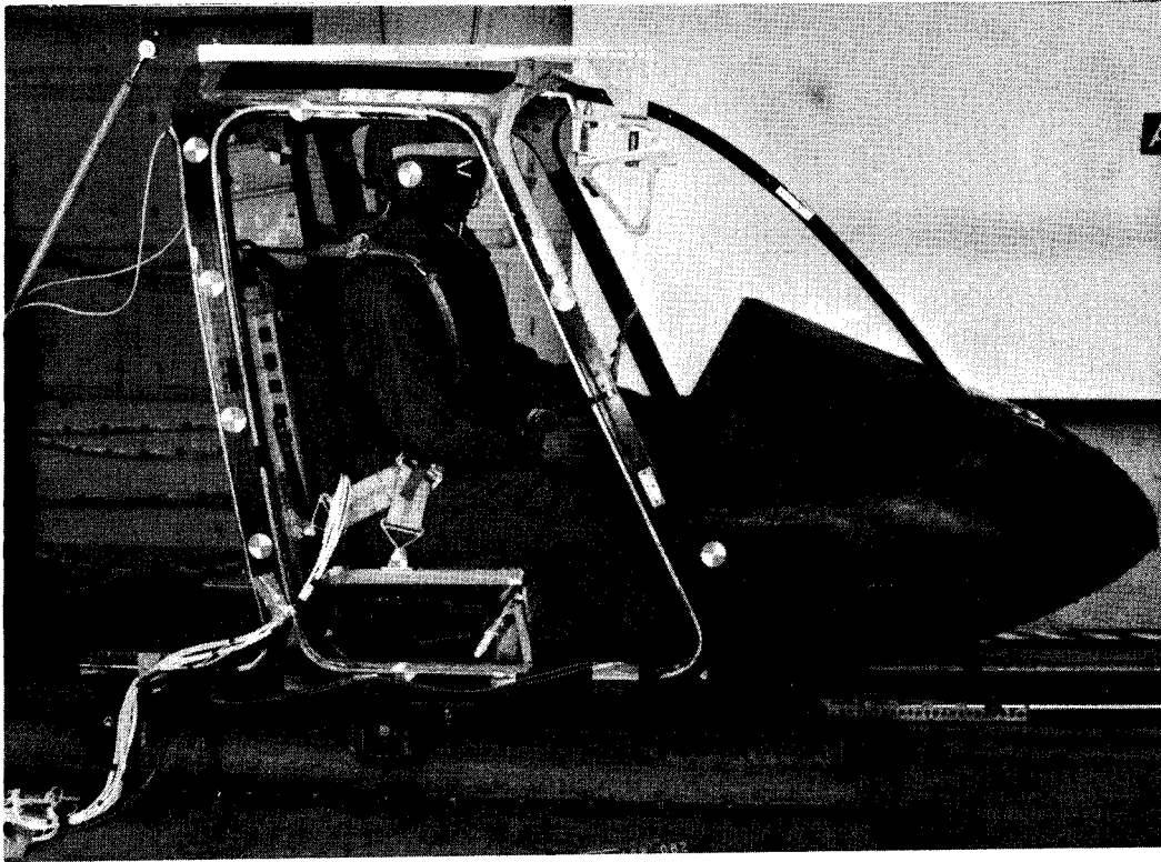
Figure 12. Pretest of no. 88062; note potentiometer cable attached to back of helmet.
