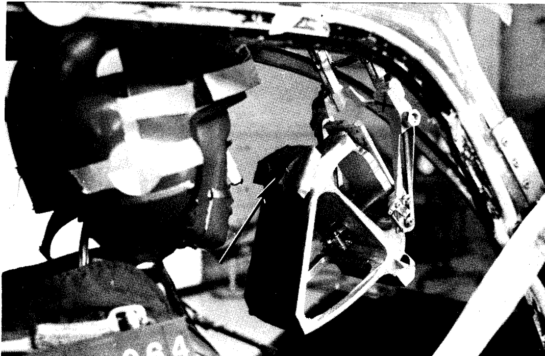
Figure 24. Posttest view of no. 88064; note detached PDU "breakaway" mount and cracked foam at back edge of PDU.
