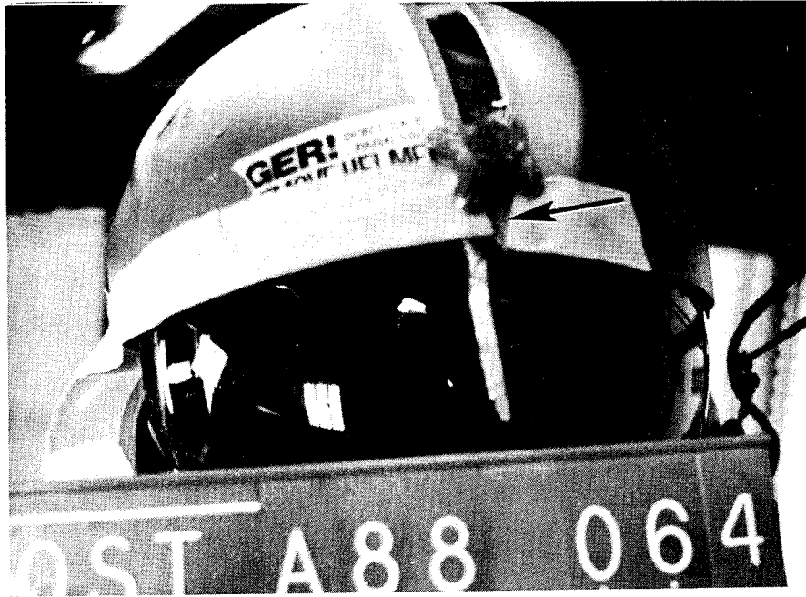
Figure 25. Posttest view of no. 88064; arrow denotes cracked helmet visor cover.
